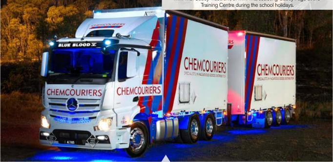
Chemcouriers Brisbane's custom-built local truck and trailer with the same capacity as a semi but with segregation advantages.
