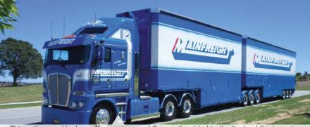
This unit, owned by Leon Thorpe, is one of 2 recently added to the linehaul fleet running between Sydney and Melbourne. The technology is the latest available with electric mezzanine floors, 190m³ and 34.5 tonne carrying capacity.
